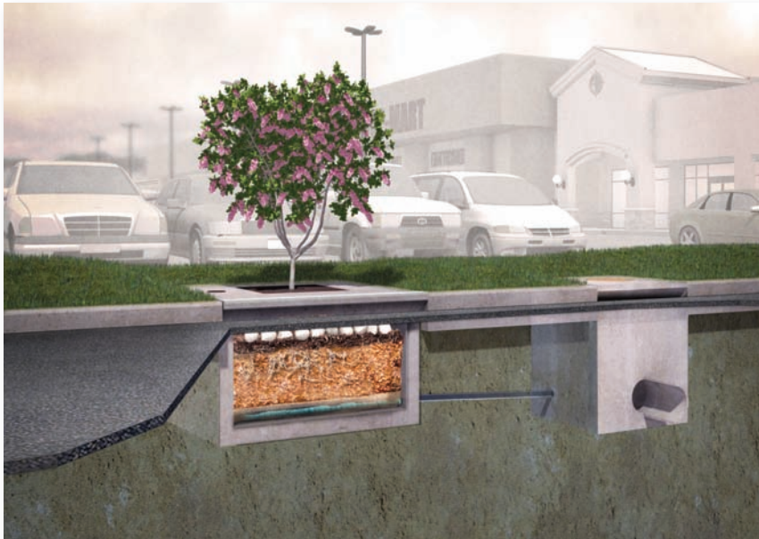
Figure 2. Filterra® / Bacterra™ Advanced Bioretention Technology
